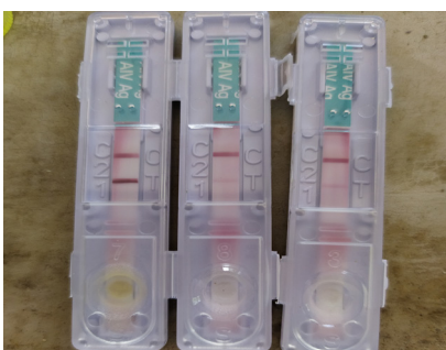
Fig-228. AIV Antigen Rapid Test; Positive with band formation in both T and C region
